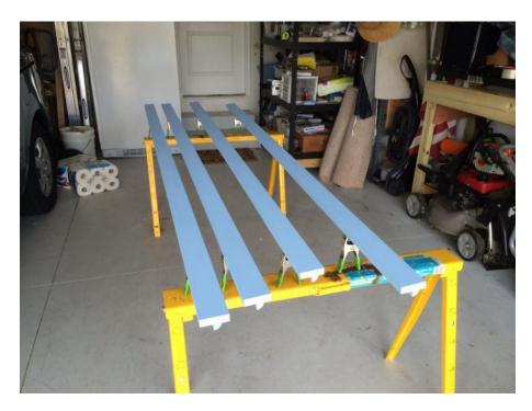
I used #6-1/2" screws to mount the boards and used a hand screwdriver instead of my drill as I didn't want to risk over driving the screws and cracking a board. I used a carpenter's 45 degree framer tool to make sure that the boards are as close to 45 degrees as I could get them.
